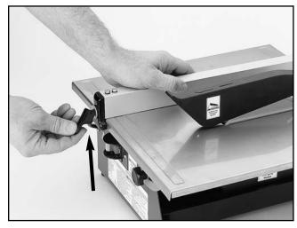
Figure 7. Rip fence locking lever.
